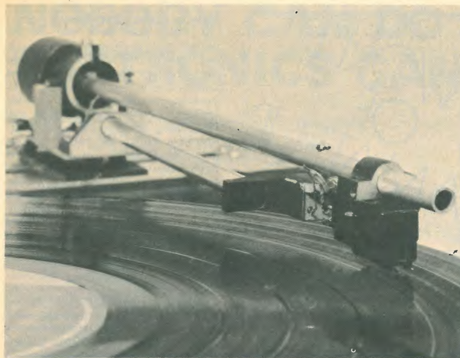
First constructional methods are not necessarily the best. Dual-purpose light slit with cue-bar to raise pickup arm (above) could be simplified; and author found simplifications could be made to the hinged platform, pivot pillars and gymbal, shown right and below (improvements in part 2).
