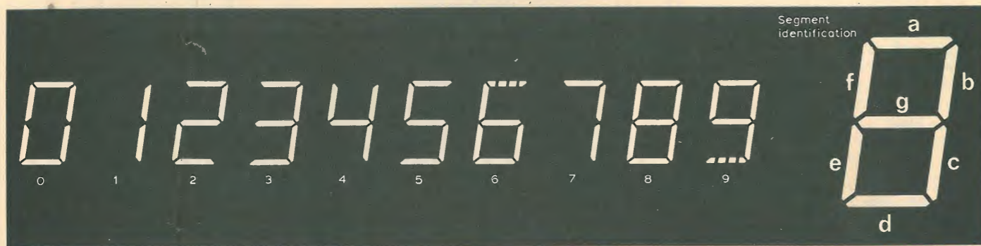
Fig. 1. Seven-segment displays of the decimals 0 to 9. Segment A on decimal 6 and segment D on decimal 9 are normally included.
