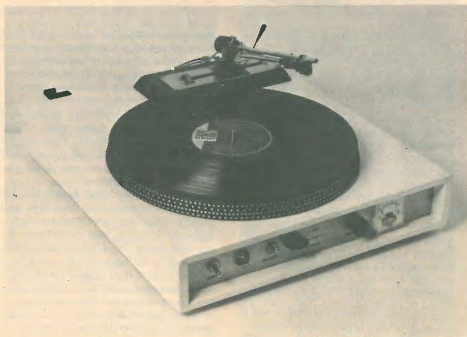
Arm is cued by lowering hinged mounting platform; see part 2 for details. Meter is an essential part of design and indicates correct operation of the servo.
