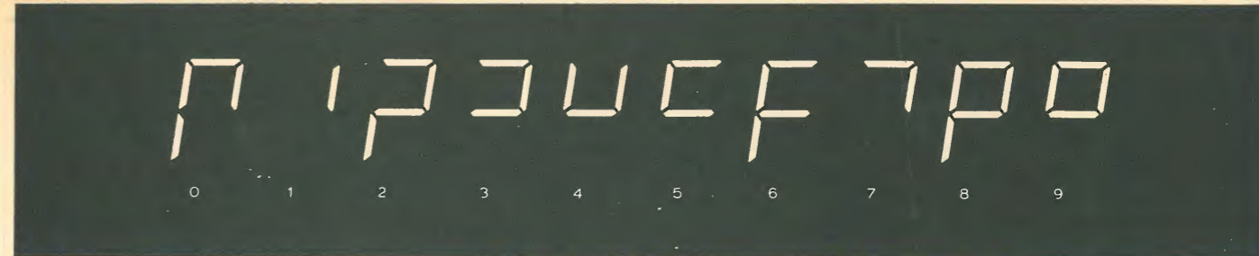
Fig. 3. Displays of the decimals 0 to 9 with both the C and D segments omitted. There are still ten distinct patterns and no confusion between the decimals.
